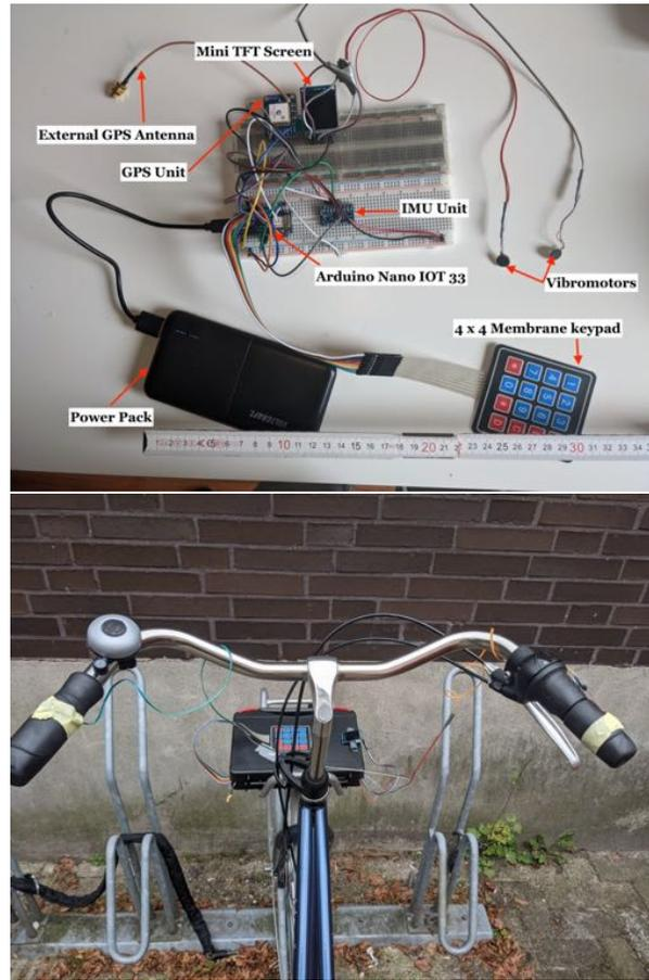
Fig. 2. (a) Hardware assembly on breadboard. (b)Hardware assembly on Bike.
